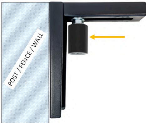
3. Take the inside point of this guide roller, and transfer its position down to the concrete - from this point, measure 30mm inwards (towards property) and mark this point as the center line for your track and run a string line or laser to identify this point at the closing and full open points of the gate. *Do not fix track yet though - following the next steps first.*
